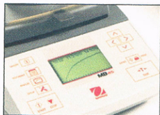
Display shows % moisture, % solids, weight, time, temperature, drying curve and more.
